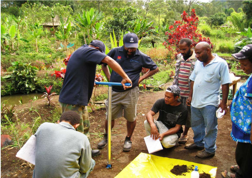
Figure 1: Soil sampling at A1 trout Farm, Goroka. The team members gained skills in selecting and using different soil sampling equipment for various soil types.
