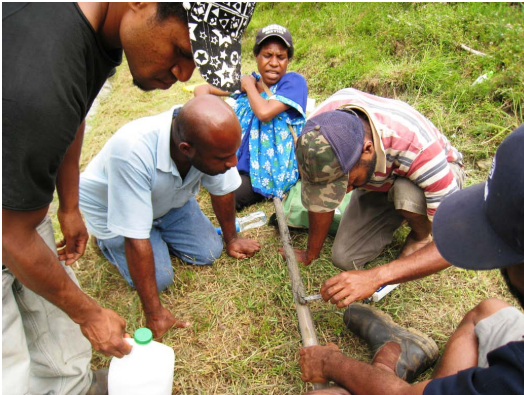
Figure 2: Workshop participants assessing soils at the Bihute Prison aquaculture ponds in Goroka, May 2009. The participants learned to extract soil cores and perform field tests on the physical and chemical properties of soil.
