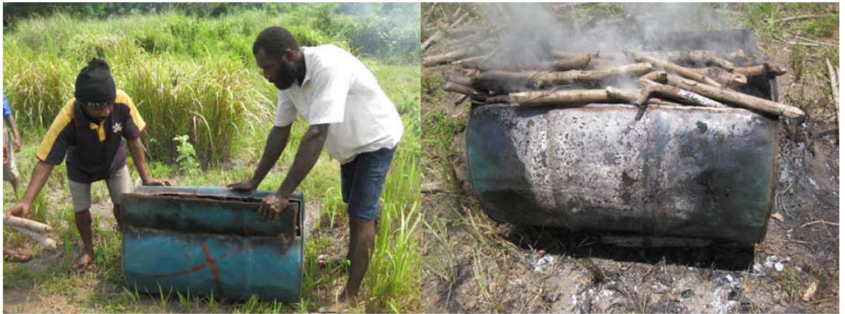
Figure 11.3.4: Topping up the last lot of woods.
