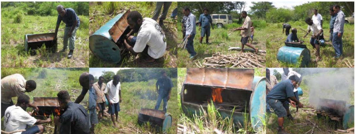
Figure 11.3.2: Process of setting up the drum and starting the fire.
