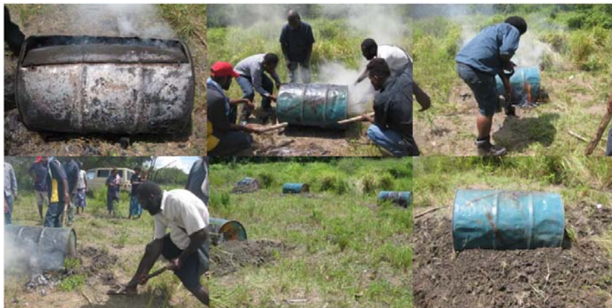
Figure 11.3.6 Sealing up the first drum, turning it over and covering it with soil.
