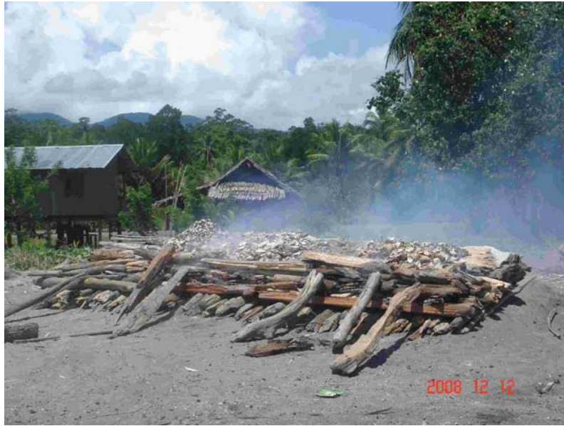
Figure 23 Lime burning under way, Morobe coast (Photo: M.Tavune)
