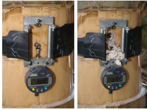
Figure 3: The French method: CIRAD-Foret strain gauge positioned on the stem of E. nitens before and after drilling the hole.
