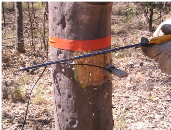
Figure 2. The German method: the HBM Type DD1 extensometer strain gauge in position on the tree stem while cuts are made to release growth stresses.
