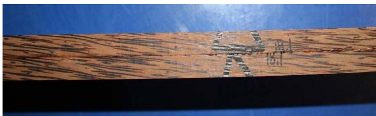
Plate 7. Split, inside reversed- top layer replaced under bottom layer
