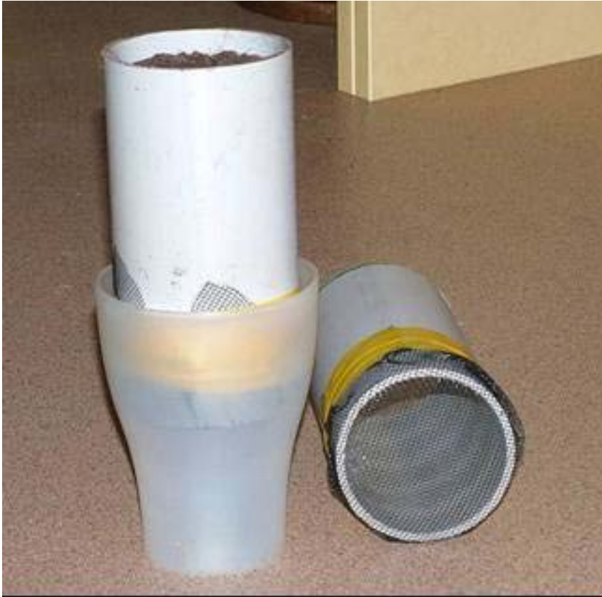
Plate 9. Water retention efficiency trial with ground cocowood potting mix, Brisbane.
