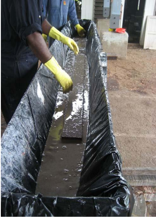
Plate 5. Anti-sapstain dipping treatment, Fiji Islands.
