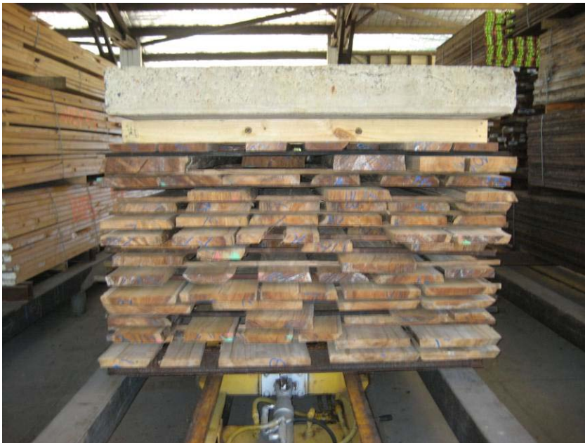
Plate 14. Sawn timber stack loaded with concrete weight to retain flatness.
