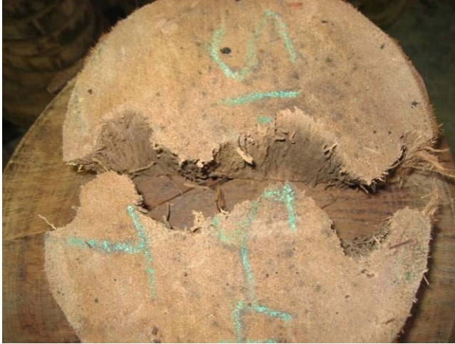
Plate 10. Grain angle variation within one coconut palm after splitting a disk.
