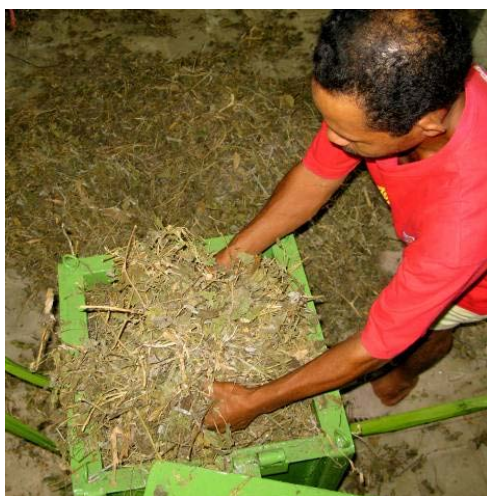
Figure 47: Legume biomass being placed into the compression box of the hand operated hay press.
