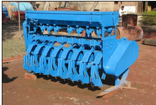
Fig. 16. 2nd prototype unit of FMI Rocket Seeder residues
