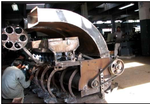
FIG. 8 Fabrication of FMI Seeder at SML factory.
