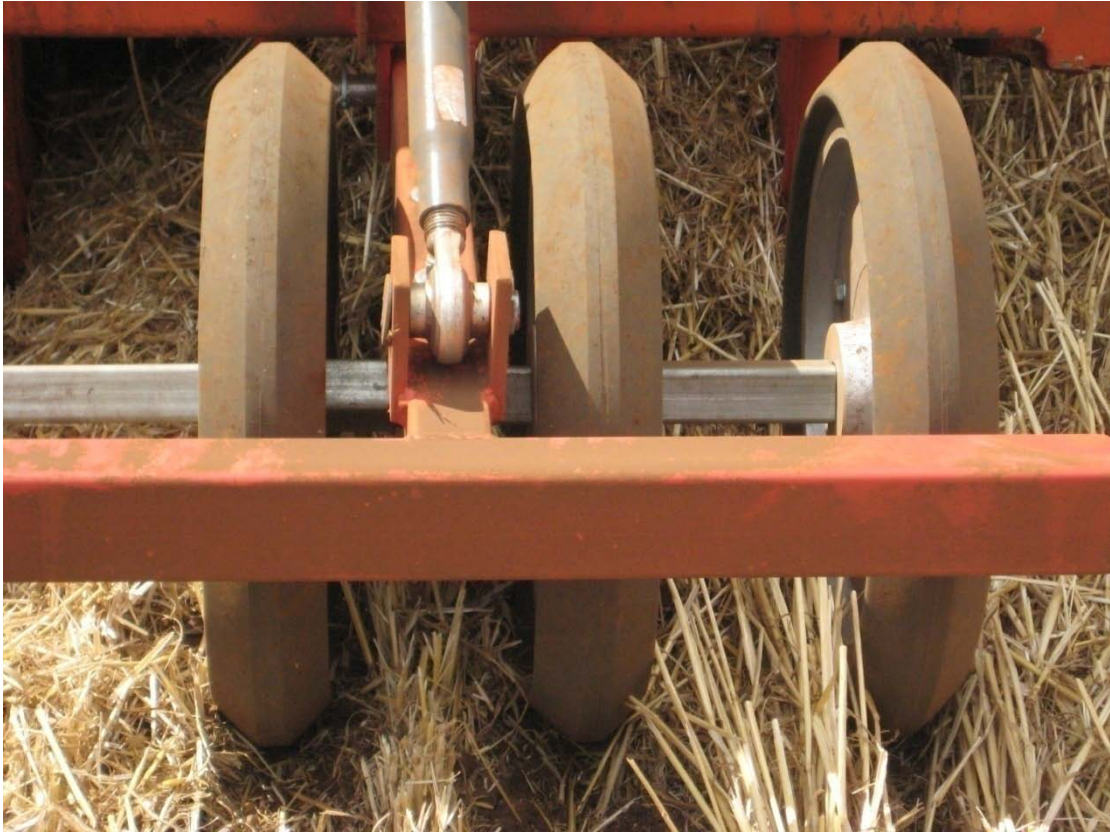
Figure 32. The press wheel and depth wheel assembly
