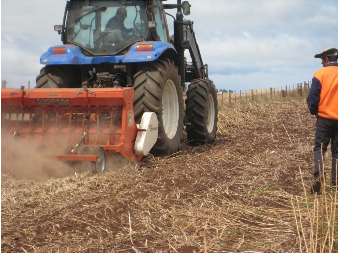
Figure 35. A full windrow of Poppy stubble poses no obstacle to the machine. Poppy capsule destruction was satisfactory, according to Poppy growers present.
