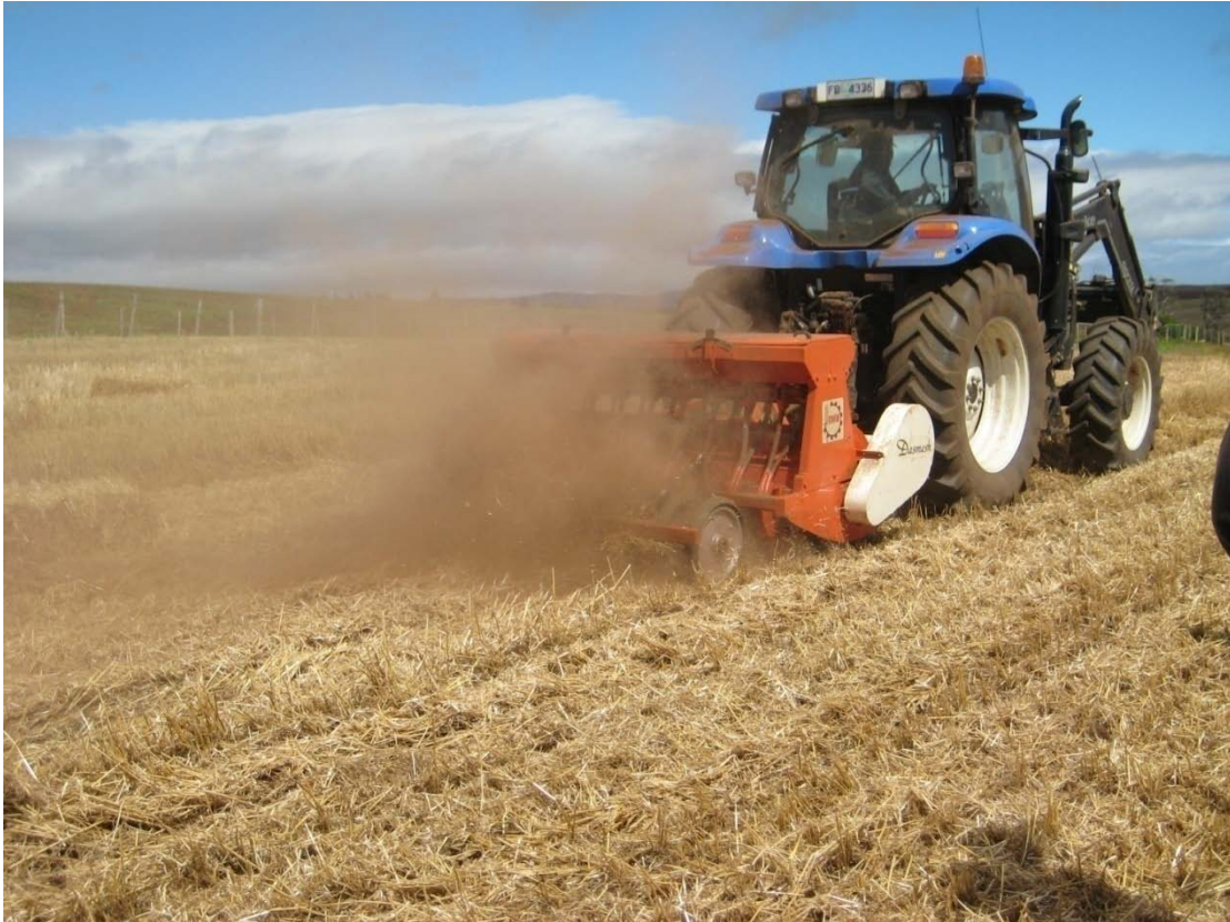
Figure 33. The modified Turbo Happy sowing into heavy Buckwheat
