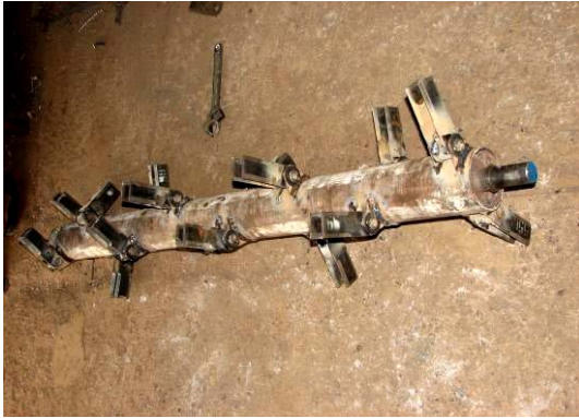
Fig.14 Knife configuration on new rotor
