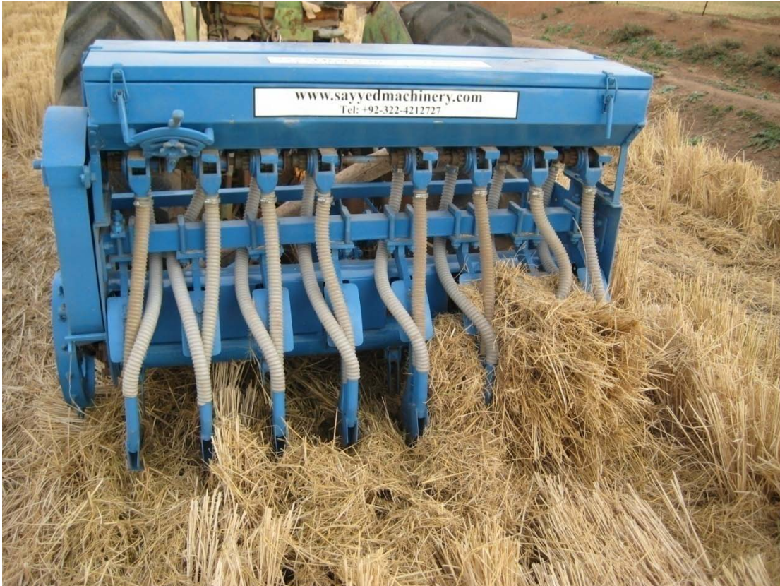
Figure 29a. The imported Rocket Seeder at normal speed in the totally rolled “laneway” of Dick Thompson’s 11.8t/ha rice straw crop.
