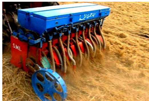
Fig.17. FMI Rocket Seeder working in heavy rice residues
