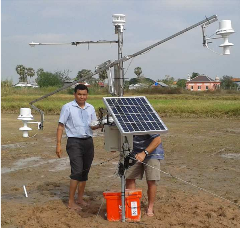
Figure 5-9 Installation of bowen ratio system at the CARDI experimental field station
