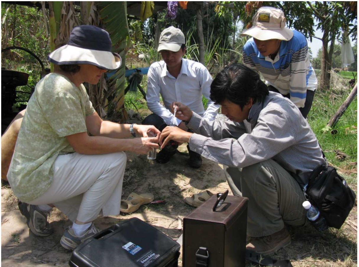
Figure 5-1 Using the Horiba 10 water quality meter and Orbeco field spectrophotometer to determine water quality parameters in groundwater
