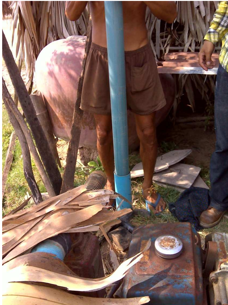
Figure 5-2 Groundwater access is via wells which comprise an inner sleeve upon which the pump head is mounted. To measure the depth using a plum line, this sleeve was taken out and the depth of groundwater was measured from the surface through the main well pipe
