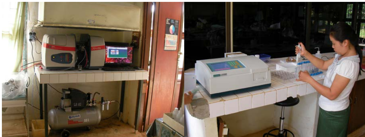
Figure 1: Installed AAS (left) and new spectrophotometer in operation (right)
