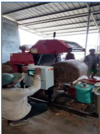
Figure 2.1.5. Mixing, pressing and packaging machine for complete feed
