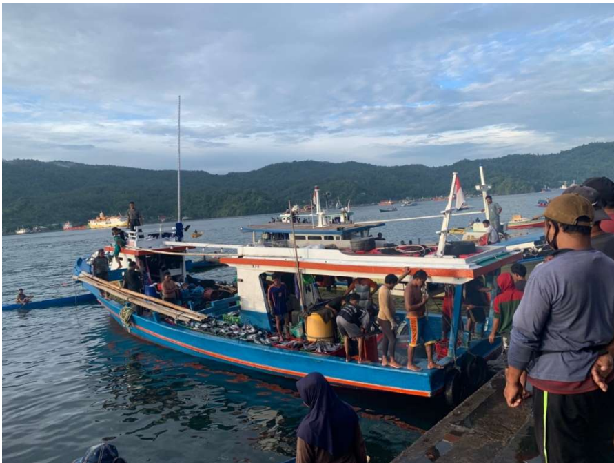
Small Purse Seine offloading at Bitung Fishing port, North Sulawesi, June 2023. Note the bamboo booms that act as surface floats for the net, and the boxes of SKJ tuna ready for offloading.
