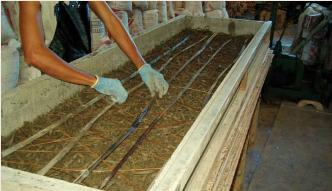
Manufacture of reinforced wood-wool cement-boards at EARN Corp., Bay, Laguna.
