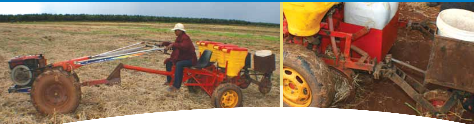
Figure 19. No-till disc planter sowing into brachiaria grass mulch. (right) Close-up of disc tyne and press wheel.
