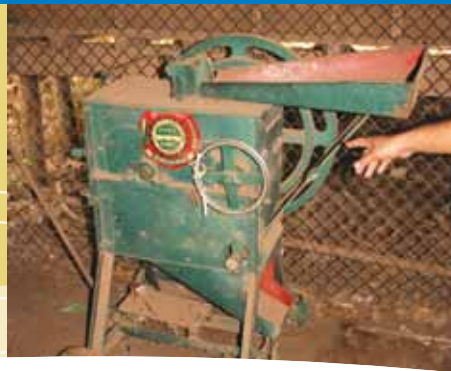
Figure 43. Portable hand-thresher for maize Photo. R Martin
