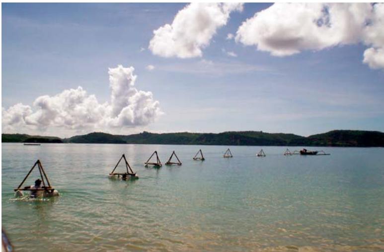
Figure 13. Experimental seed-collecting devices consisting of a bamboo-framed tripod mounted on styrofoam floats from which shelter traps are suspended
