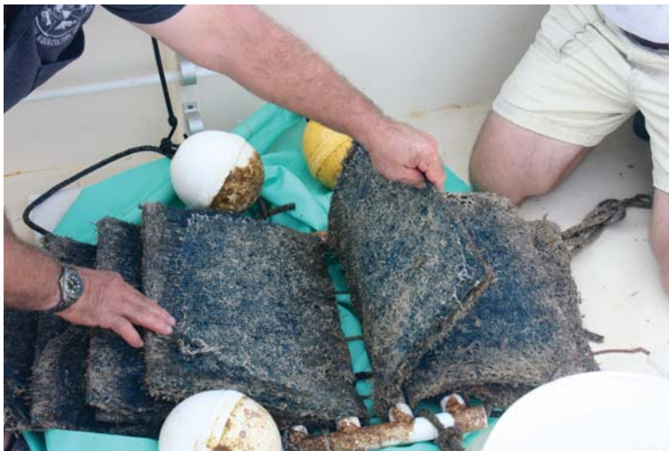
Figure 1. A modified Witham or Hunt collector being cleared of seed lobsters on the deck of a boat. The fibrous panels are air-conditioning filter material made from compressed pigs’ hair. When in water, these panels hang from a polyvinyl chloride (PVC) frame that is suspended just below the surface by the four polystyrene floats.
