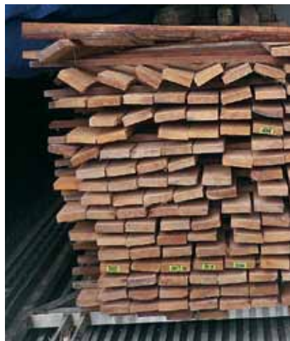
Twisted boards in an un-weighted stack
