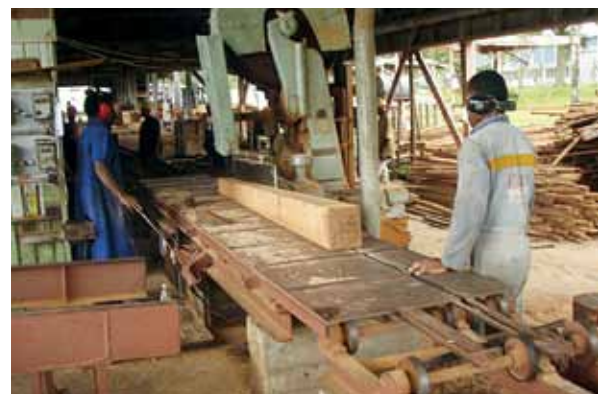
Fixed band-saw; high density boards removed
