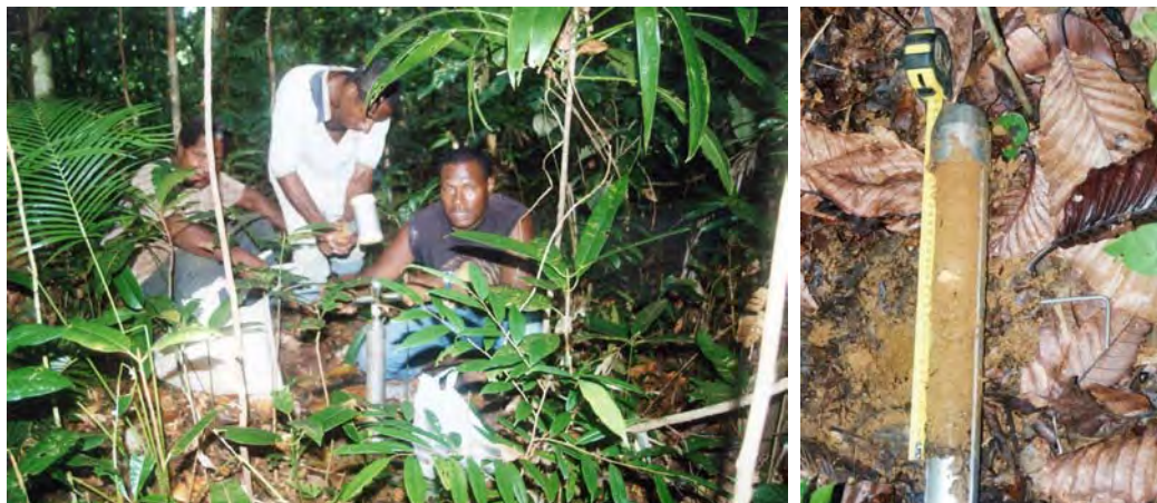
Figure 3. Soil coring using split-tube sampler
