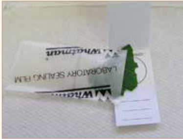
e. A piece of leaf torn to fit the card, and covered with a clean piece of paraffin film or plastic wrap to prevent contamination
