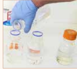
f. Adding the bleach (1.5% sodium hypochlorite)
