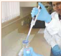
a. Adding HCl to adjust the pH of the extraction buffer (TBS plus sodium sulfite)
