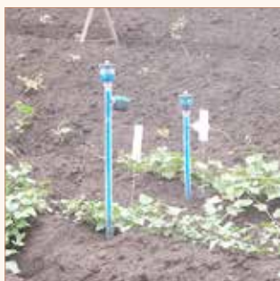
Figure 37 Tensiometers at different depths in the soil to measure water needs
