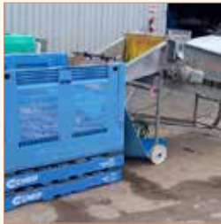
b. A small mechanical washer, which also delivers fungicide before the roots are drained
