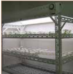
h. A simple metal-framed bench with fluorescent lights at the top connected to a timer. Note: unless lights are placed above each shelf, the lower shelves receive less light
