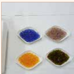
g. Different colours of silica gel before and after drying: purple and orange when dry, and pink and green when moist
