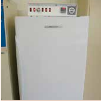
a. A converted refrigerator, which is factory fitted with four fluorescent lights built into the door, a heater, and a control panel to regulate heating and cooling, and to set times for the lights to turn on and off
