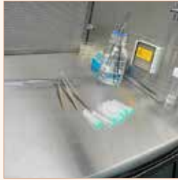
b. Instruments in alcohol, sterile hypodermic needles in plastic covers, and medium in 30 mL plastic bottles ready to receive meristems
