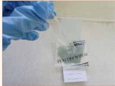
f. Transferring the leaf contents to the card by gently rubbing a test tube on the surface of the paraffin film
