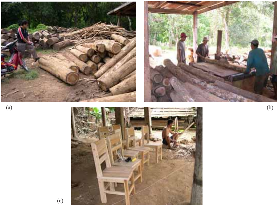
Figure 3.1 Small-scale processing of teak. (a) Logs awaiting milling; (b) A typical sawmill; (c) Village-level manufacture of chairs
