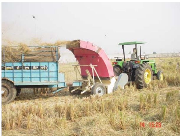
Figure 4. The straw handling unit of the Mark 1 Happy Seeder with modification for harvesting rice straw into a trolley
