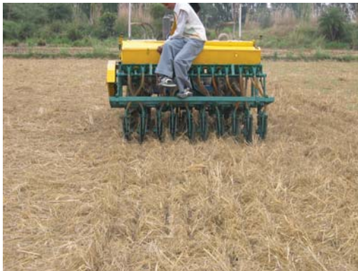
Figure 2. Double-disc drill for seeding into loose residues
