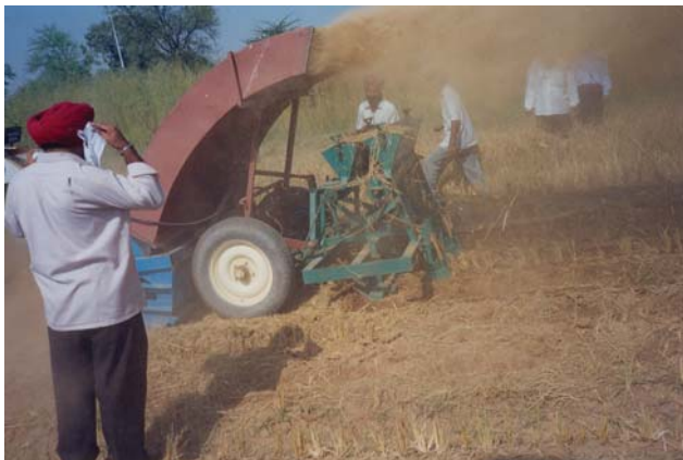
Figure 2. The first Mark 1 Happy Seeder with bed planter, sowing wheat into rice stubble on beds in October 2002
