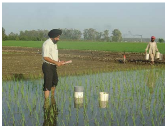
Figure 1e. S.S. Kukul with PVC cylinders used for measuring infiltration in puddled transplanted rice with continuous flooding (PTR-CF) in a small plot on loam soil in 2004
