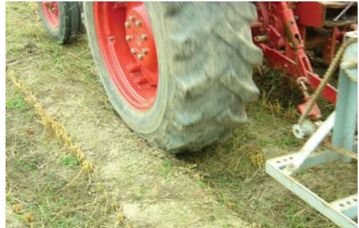
Figure 17. Tractor wheels pressing on location where rice is transplanted (rows of rice stubble) on sides of beds
