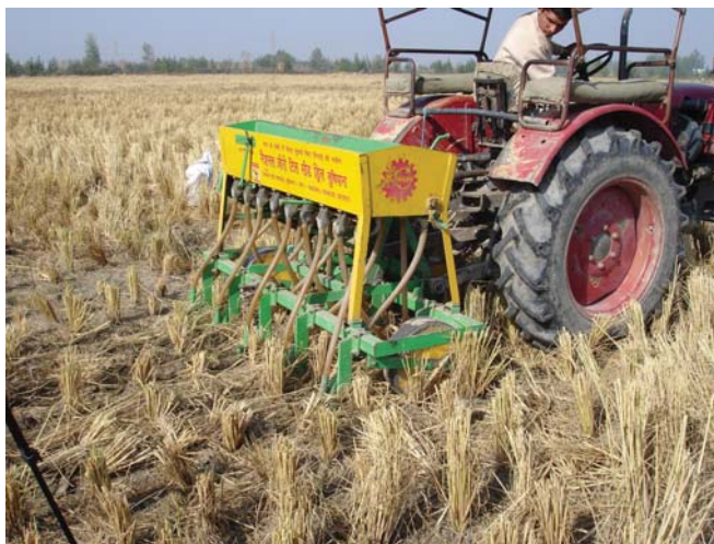
Figure 1. Zero-till drill used for creating slits for transplanting rice
