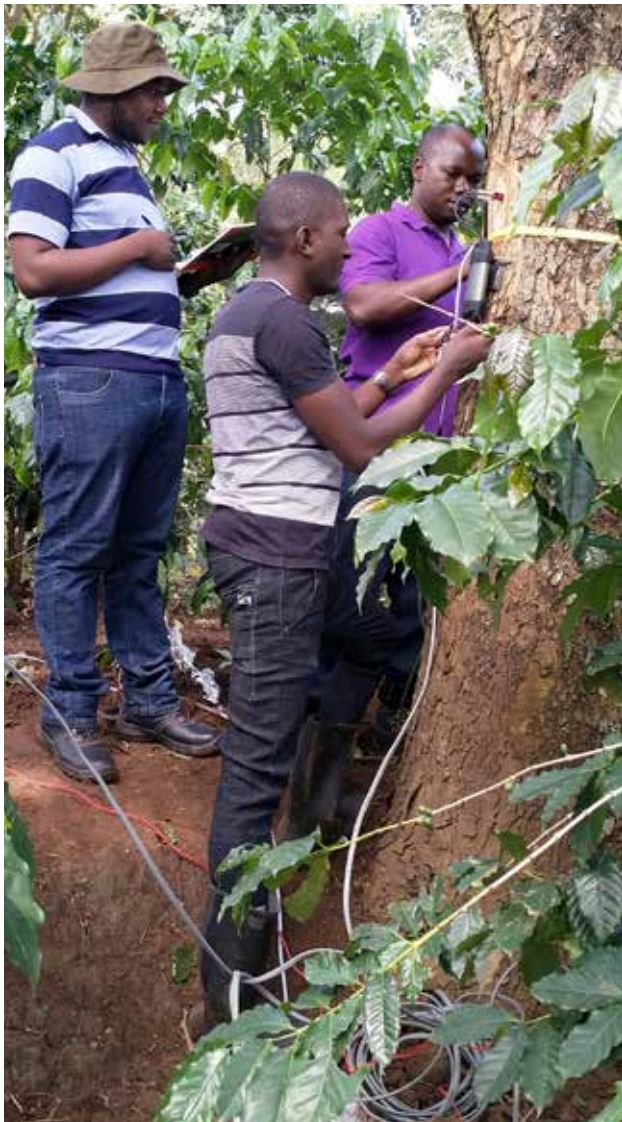
A research team installing a sap flow meter and collecting tree meta data from an Albizia tree growing in a coffee plantation. Photo: Joel Buyinza. ACIAR project: FST/2015/039.
