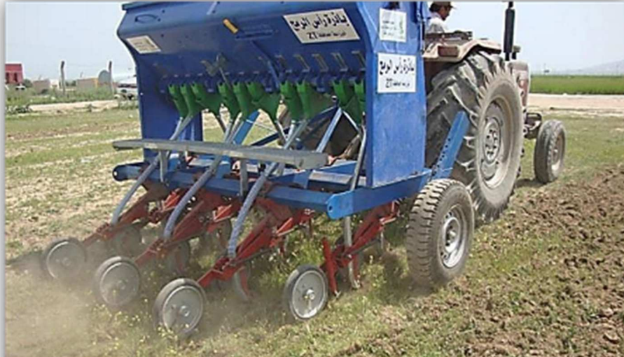
Fig. 4: The second Ras Alrumh seeder prototype being tested in Mosul in 2014.
