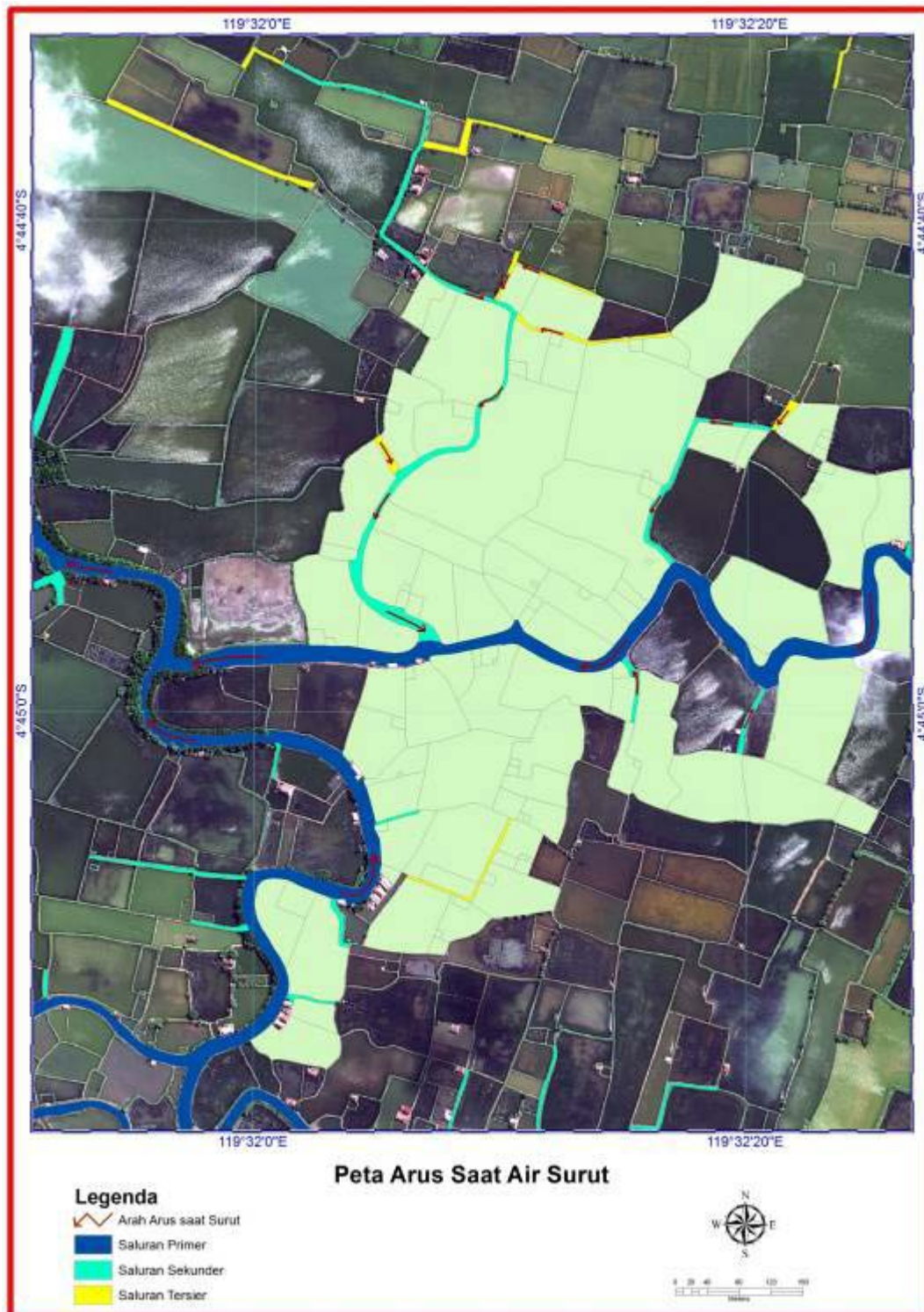
Figure 8: Map of canal structure at study site including water flow at low tide
