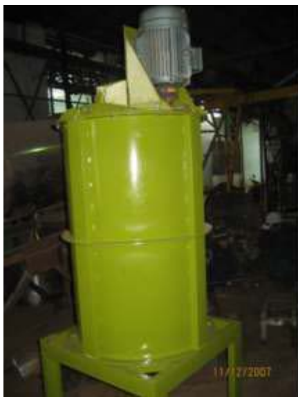
Figure 8.3 specifically engineered water homogenisation equipment for processing rubber seed to maximise HCN release from the seed
