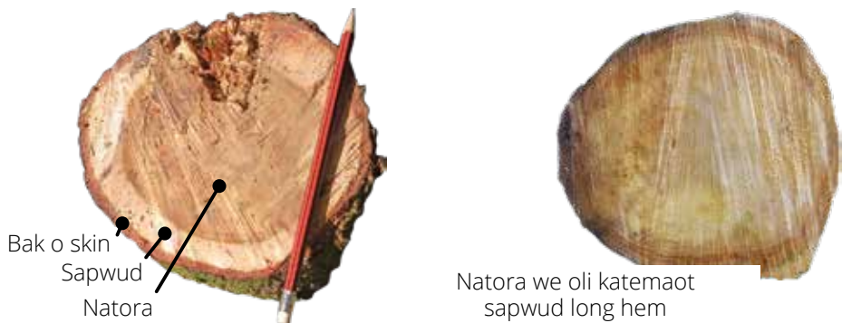
Figia 10.3 Kros-seksen blong sandelwud log (lef saed) i soem skin, sapwud mo natora; mo (raet saed) i soem natora afta we skin mo sapwud i kamaot.
