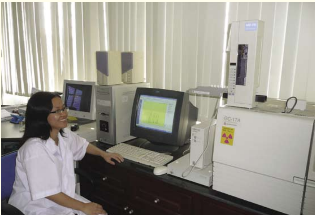
Current trainee Ms San Trân Anh surveys a pesticide chromatogram on the SIAEP's ECD gas-liquid chromatograph.
