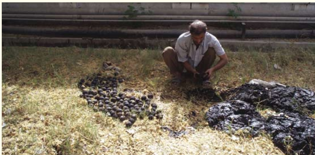
A worker preparing 'cannon balls' from the Sirolan CF sludge for incineration trials at an Indian mill.
