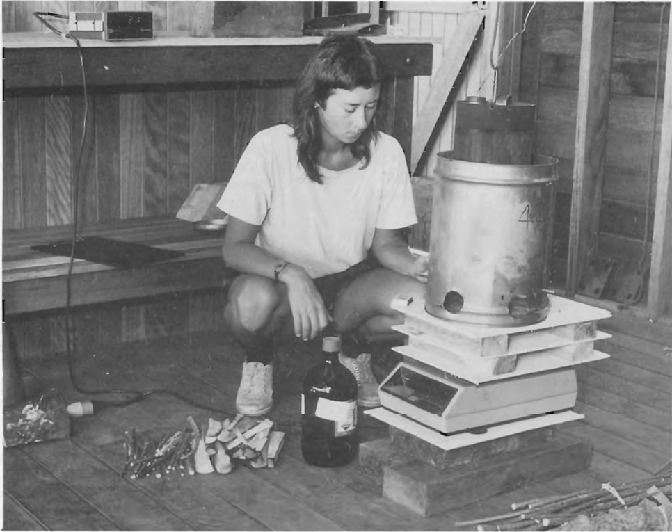
Fuelwood testing unit developed by the Queensland Department of Forestry. Robyn Bell is shown with the test rig, consisting of a weighing balance, protective asbestos sheeting, a small drum to contain the fire and another small drum containing water inside the fire drum. The temperature of the water is monitored. Photograph courtesy of the Queensland Department of Forestry.
