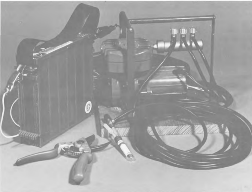
Plate 4.2 Equipment used to vacuum-extract xylem sap from stems. Diaphragm vacuum-pump with manifold and three vacuum lines, rechargeable 12 volt battery, secateurs, Vacutainer and fittings.
