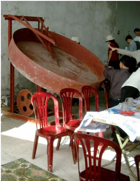
A BioGro mixer installed in the Hoa Lac factory in Ha Tay province
