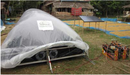
Fig. 4. Solar bubble dryer (left) and farmers method of sun drying (right).
