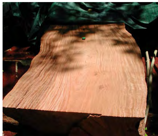
Sawn buttress of P. indicus showing attractive flame figure; Espiritu Santo, Vanuatu (Photo: L. Thomson)
