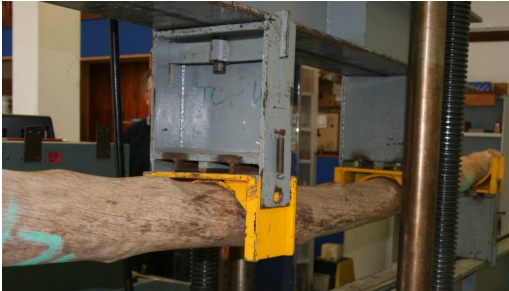
Plate 9. 20-year-old Solomon Island poumuli pole under test for MOE and MOR.
