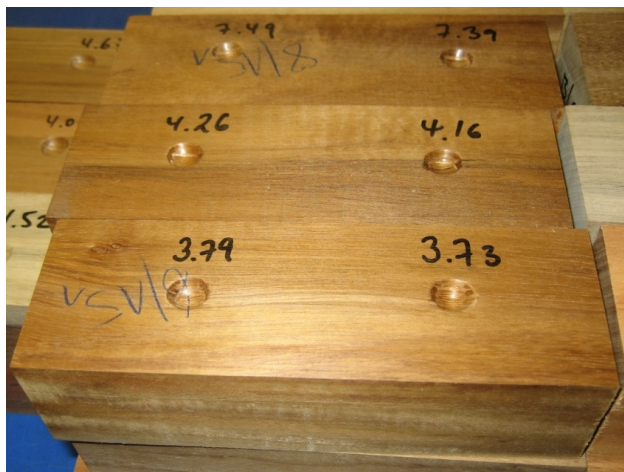
Plate 5. Specimens after test, showing indentation.
