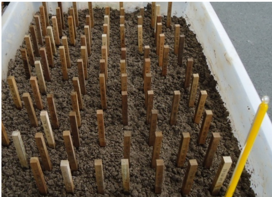
Plate 6. Accelerated mini-beam durability indicator test.
