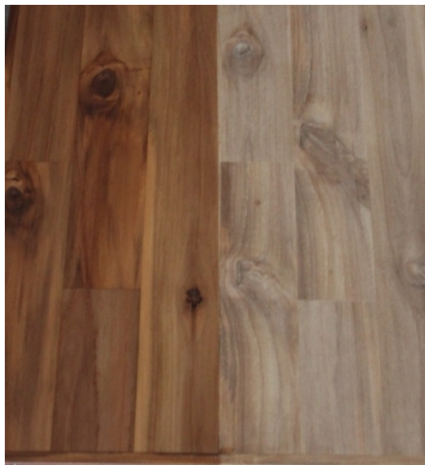
Plate 12. Knotty grade Solomon Island plantation teak flooring (left half with clear finish coating, right side unfinished, natural).
