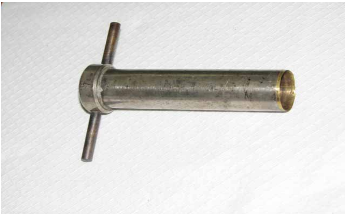
Figure 2. Cork borer used to remove the endosperm plug from the split nut.
