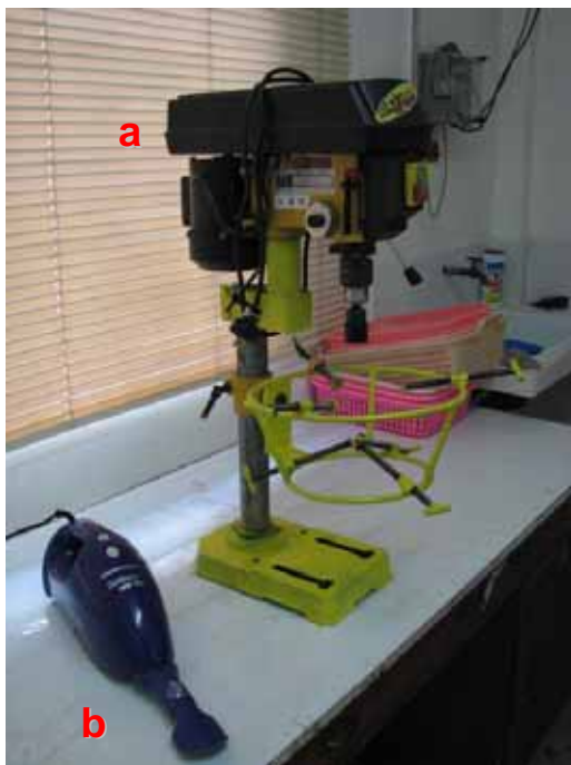
Fig 1. a) Bench drill with attached nut holder, b) Hand vacuum cleaner
