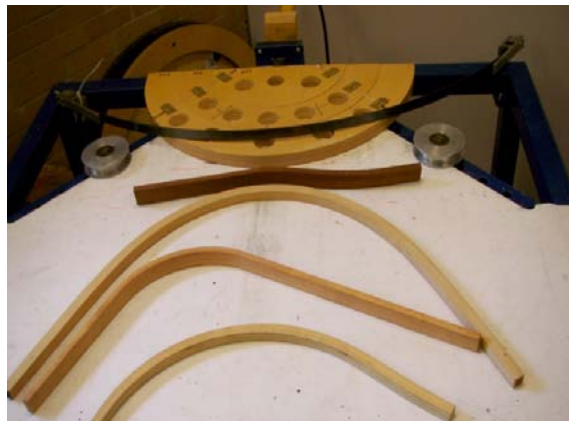
Figure 10: Wood bending rig under construction at Pakpasak Technical College
