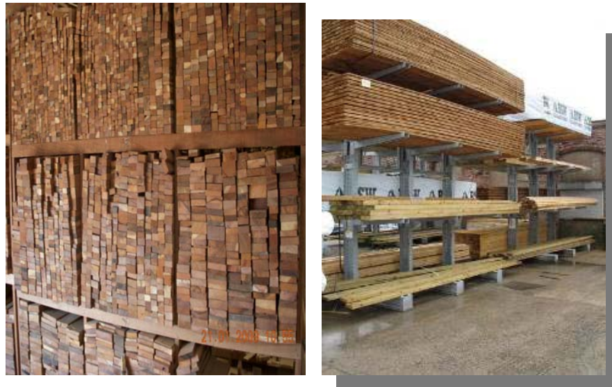
Figure 7: Improvements in wood waste management through segregation of timber into sizes and proper storage conditions.
