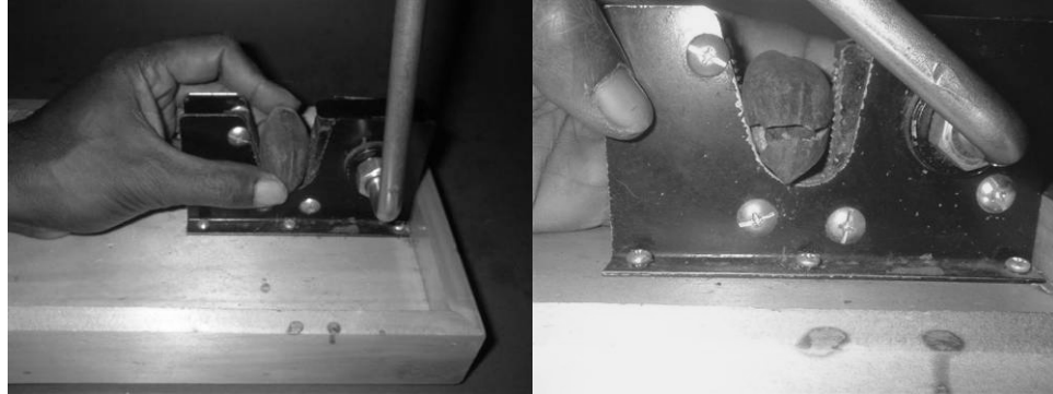
Figure 1.A) The modified TJ's™ nutcracker showing the orientation of the Canarium indicum nut flat side up and B) the fracture along the germination suture when pressure is applied from the jaws of the cracker.
