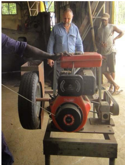
Fig. 5. A mechanical dehusker developed to remove the pulp from the canarium nuts.
