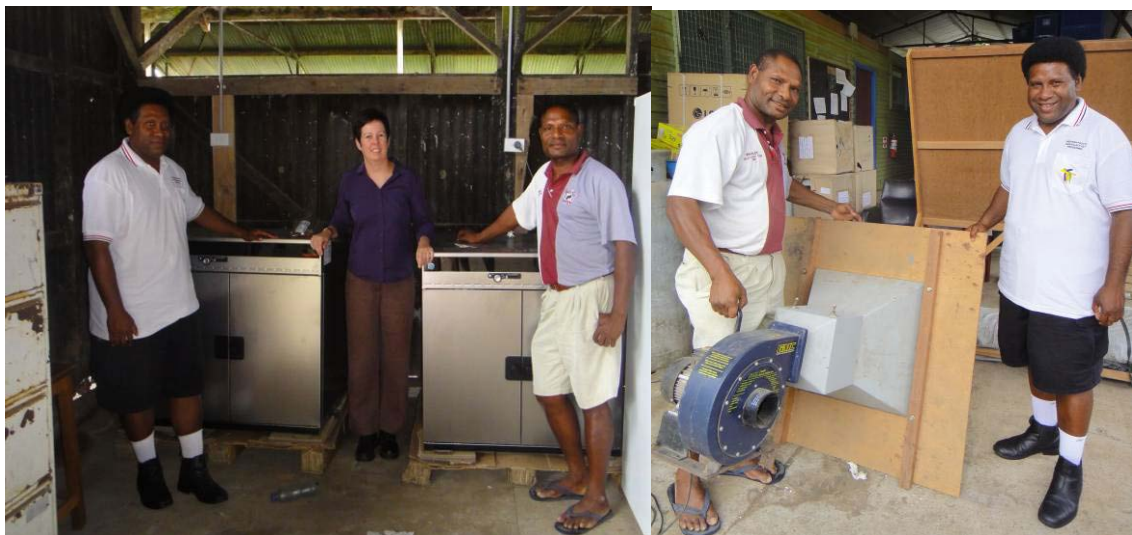
Fig. 21. (a) Scientific ovens and (b) NIS bell box drier system showing fan and hood
