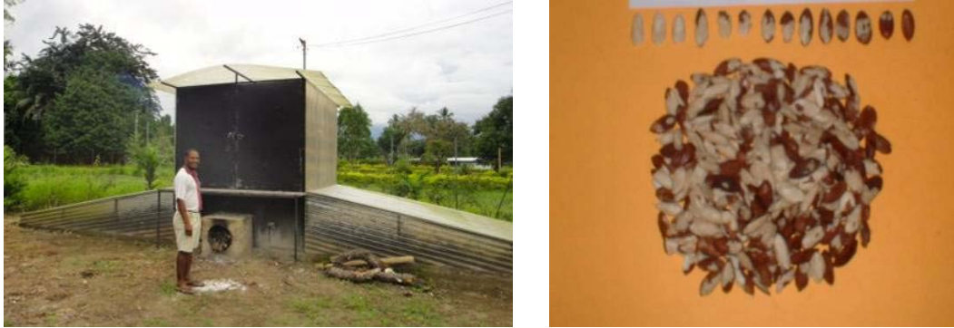
Fig. 8. (a)Solar dryer used for cocoa drying and (b) Kernel after being dried in the solar drier for 17 days.
