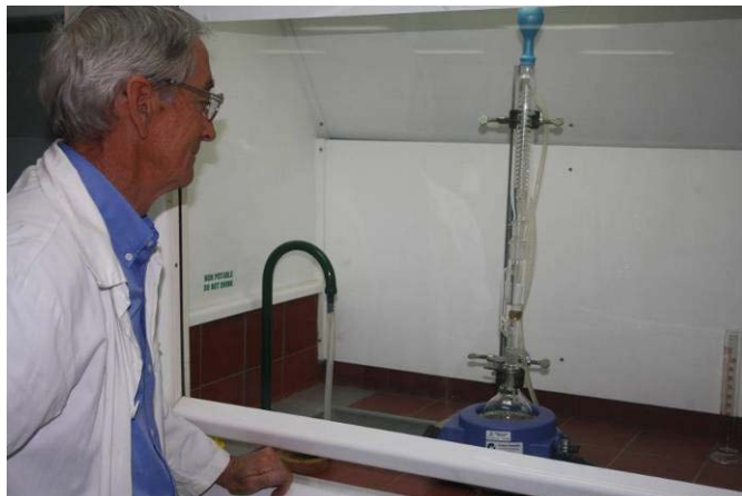
Fig. 1. Oil Extraction using a Soxhlet type extraction apparatus
