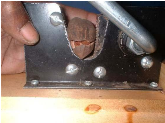
Fig. 12. The modified TJ's™ nutcracker showing cracking of canarium nuts
