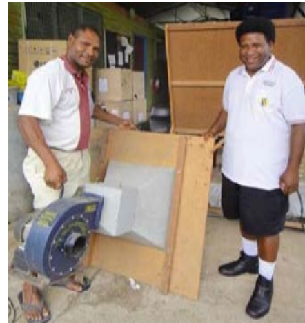
Fig.11. Bell box drier showing plywood box structure, fan, heating element and hoods.
