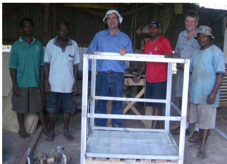
Fig.10. Metal frame and base for Bell box drier.
