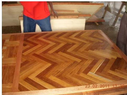
Figure 6: Research on the production parquetry flooring using PNG species
