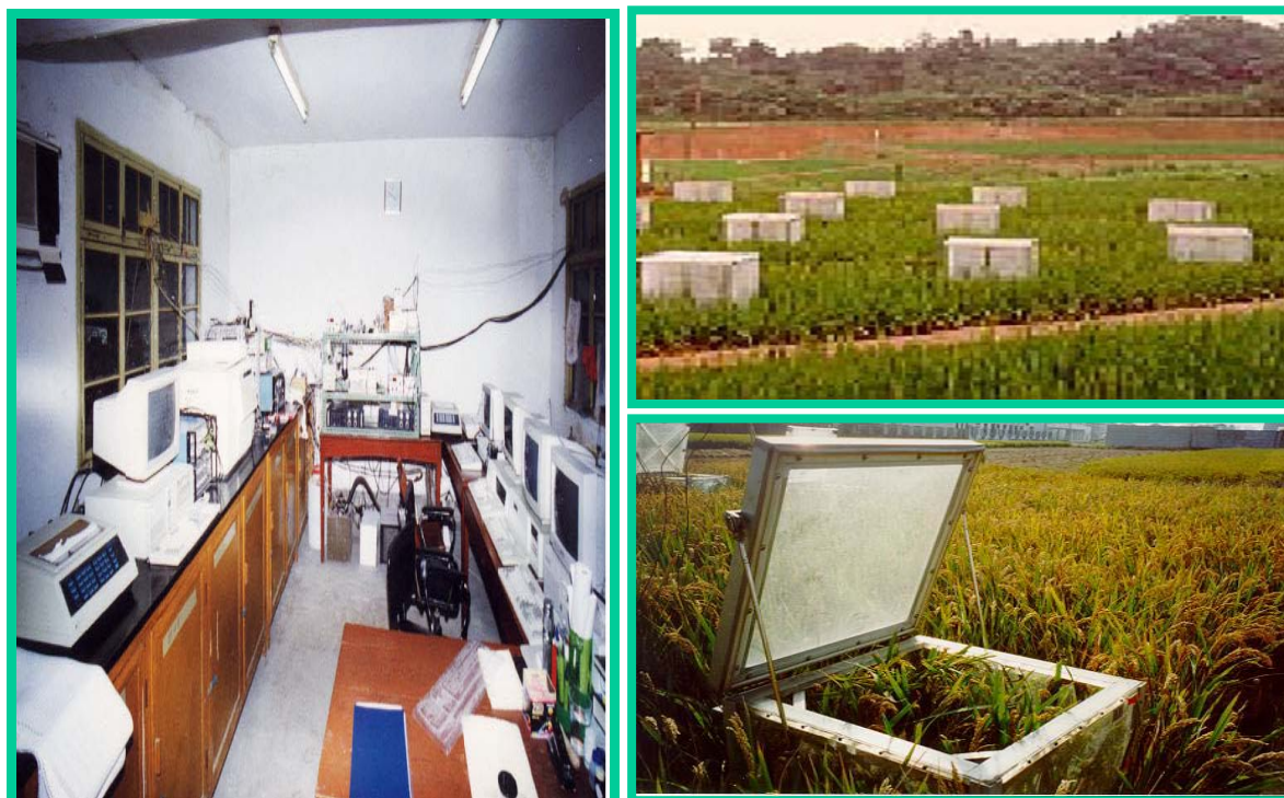
Fig. 4. Automatic chamber system at the Yongji Site, developed by Institute of Atmospheric Physics, Chinese Academy of Sciences (IAP-CAS).
