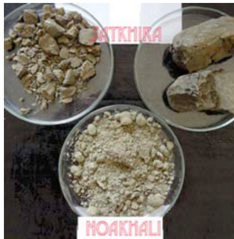
Figure 7.1 Soil of Satkhira (clay, setting like concrete) and Hazirhat, Noakhali loam, powdering easily
