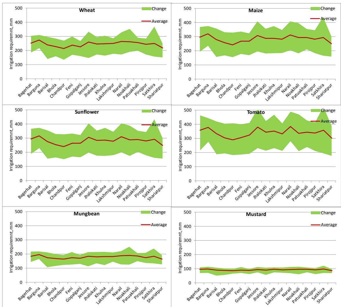
Figure 5.55 Net irrigation requirements of several species in a clay loam soil sown on 30 November
