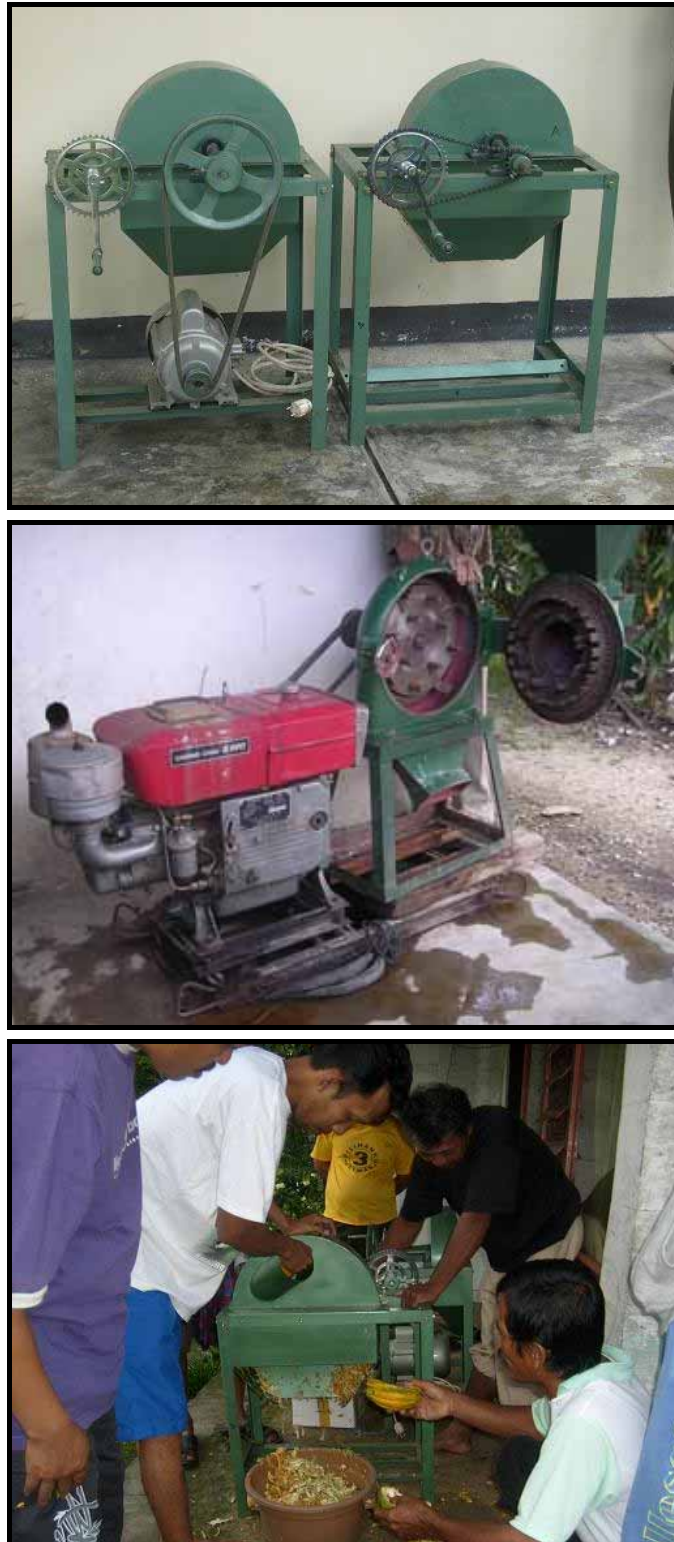
Figure 5. Electric (upper, left) and manual (upper, right) cocoa-pod choppers and the original cocoa-pod grinder (middle) evaluated and farmers using the new manual chopper in Ladongi sub-district, South East Sulawesi.
