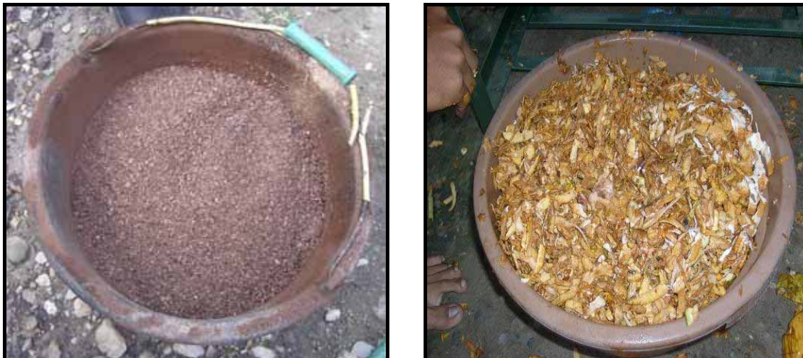
Figure 6. End-product of the cocoa-pod grinder (left) and the manual cocoa-pod chopper (right) evaluated in Ladongi sub-district, South East Sulawesi. The manual and electric cocoa-pod choppers produced a similar consistency of chopped cocoa-pods.
