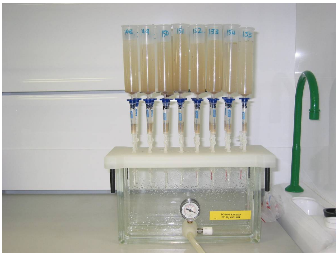
Fig. 3.1. Reservoirs connected to SPE cartridges on vacuum manifold.
