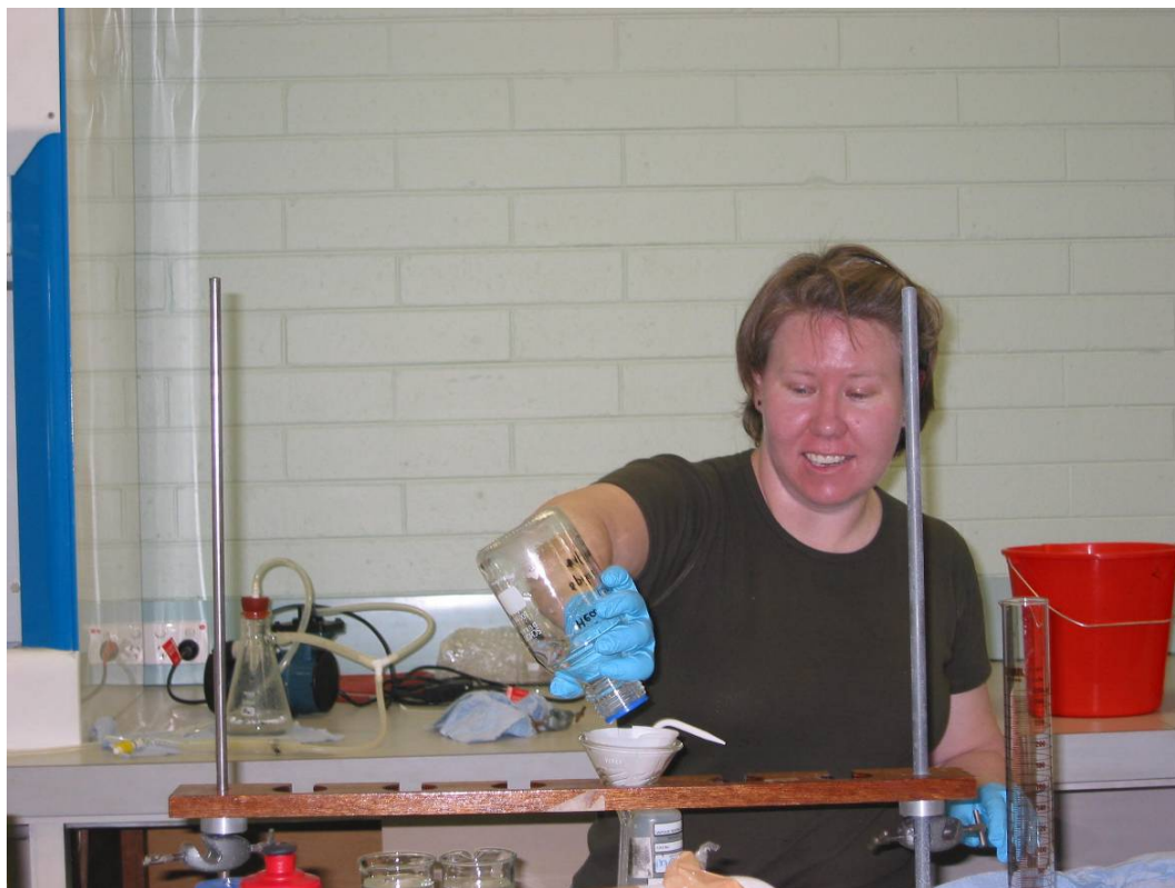
Fig. 3.2. Filtering the water sample through glass fibre filter paper to remove colloidal material.
