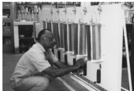
CFTRI's Mr N. Muralidharan assembling test chambers during the project, for fumigating infested grain to estimate dosage requirements for phosphine.
