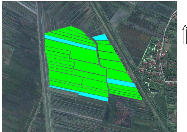
Figure 4. 'Traditional polyculture' growout ponds (green) with crustacean-free biofilter/reservoir ponds (blue) operated by 'Windu Jaya Dua' farmer group for the 2009 outcomes study trials.
