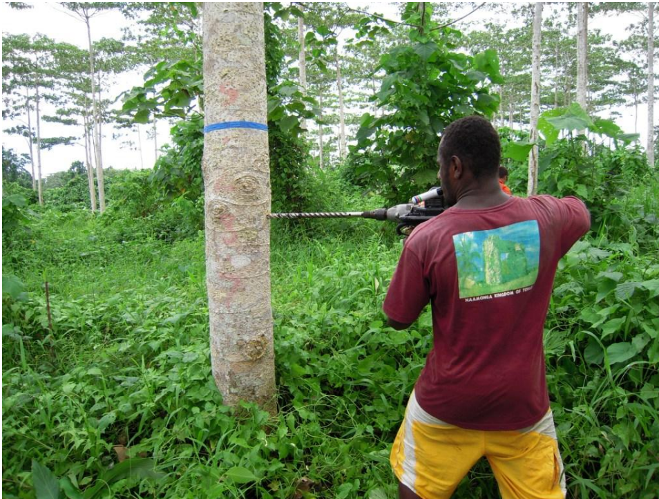
Figure 4 Taking wood core samples from IFP seed orchard to compare wood density of different whitewood families.
