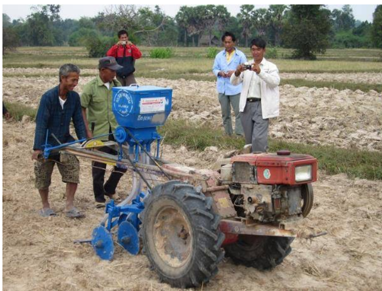
Figure 2: The Thai-built, disc-based direct seeder used in the farmer demonstration trials in western Savannakhet
