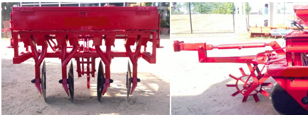
Figure 14: The modified Brazilian, disc based, dry direct seeder being manufactured in Pakse, Lao PDR
