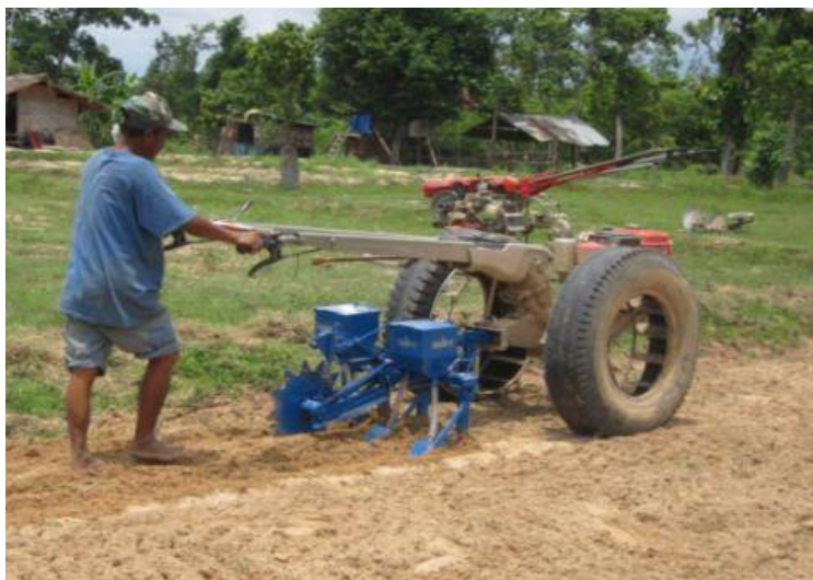
Figure 13: The smaller, lighter, tine-based Thai seeder trialled independently by farmers in Savannakhet in wet season 2013
