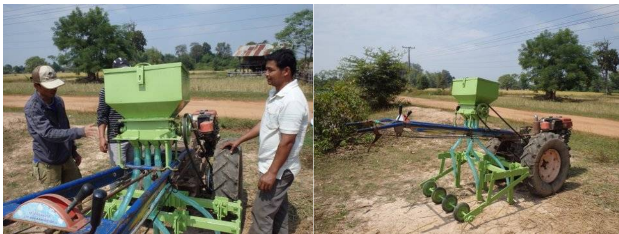
Figure 4: The modified, tine-based Thai seeder with dual seed and fertiliser box trialled by farmers in Savannakhet in wet season 2014
