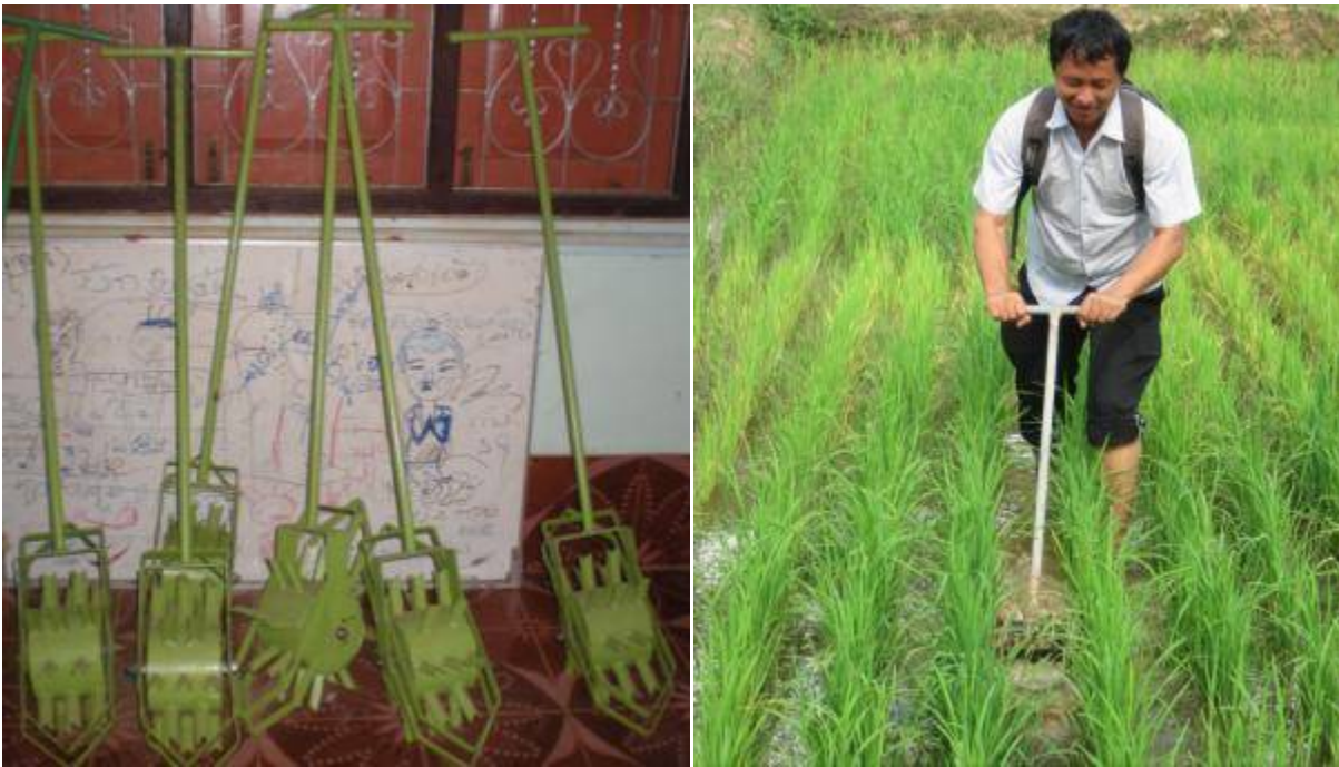
Figure 12: (left) Rotary weeding tools; (right) Mr Lytoua Chialue, a project researcher from NUOL, demonstrating the rotary weeder in Ban Sakheun, Champhone
