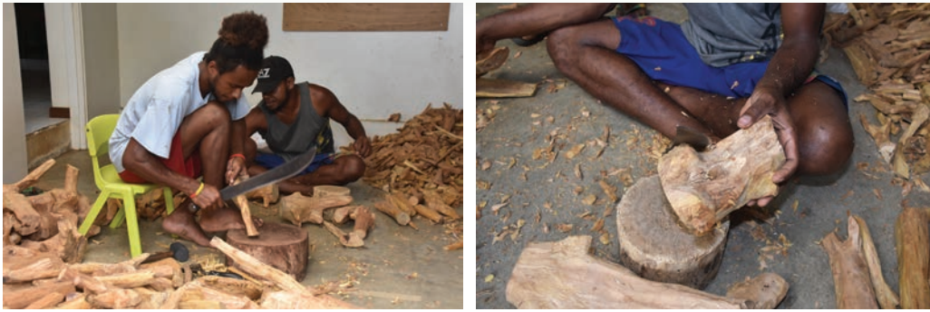
Figure 10.5 Secondary manual processing of sandalwood where all traces of sapwood are cut away from the heartwood
