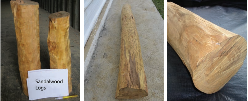
Figure 11.5 Logs – de-sapped, large-diameter sections of trunk heartwood 30–100 cm long and >10 cm diameter at smallest end
