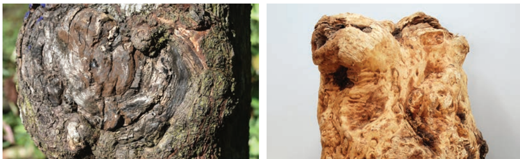
Figure 11.14 Burls are outgrowths on the stem (left) and form rare decorative pieces of wood (right)
