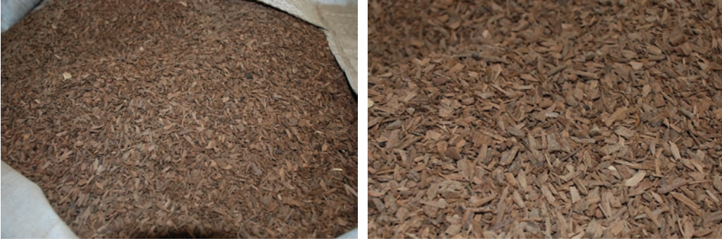
Figure 12.1 Heartwood is milled to a consistent size specification (grade) of 3–5 mm chips, which are then used for extraction of oil
