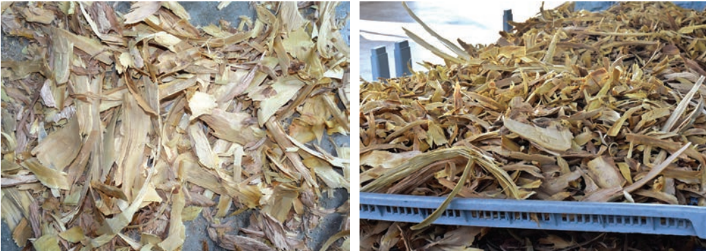
Figure 11.8 Second cutting chips – a by-product of final de-sapping after the bark has been removed; typically contains a 1:1 proportion of heartwood and sapwood
