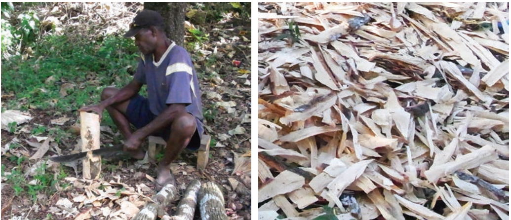
Figure 10.4 Removing after bark and sapwood (left), and the sapwood chips as a by-product (right)
