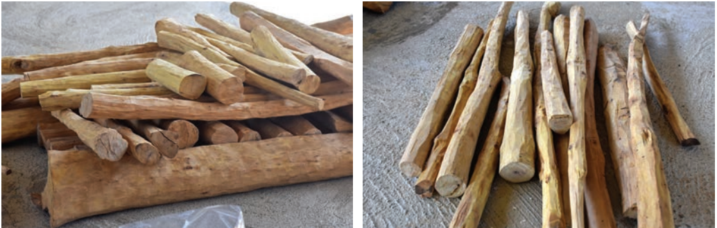
Figure 11.6 Billets – de-sapped, small-diameter sections of branch and trunk heartwood 30–100 cm long and 3.5–10 cm diameter at smallest end
