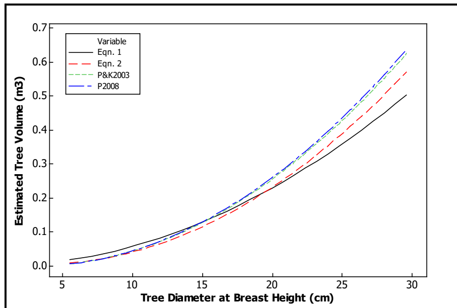
Figure 7.9: Estimated tree volume across diameter range using Equations 1 and 2 (volume under-bark), and tree volume equations for teak in Costa Rica (over-bark) published by Perez and Kanninen (2003; P&K2003) and Perez (2008; P2008).
