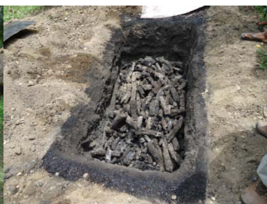
D & E] 2m 3 metre pit oven by the Wampup Ragin group, Saruan village, Kaiapit, Morobe Province; F] charcoal bags produced from the pit oven.
