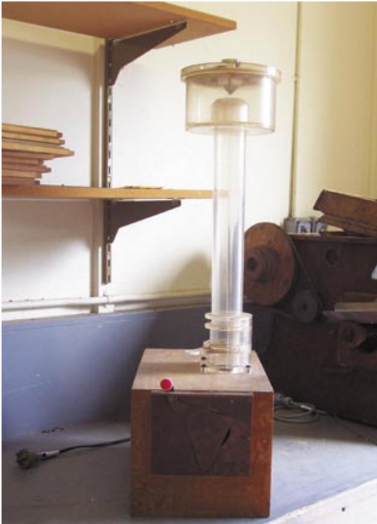
An aspirator used for cleaning seeds. Air is gently blown from a small fan in the base housing through the column, where dehusked seeds are collected in a sieve, while dust and husks accumulate in the top container.
