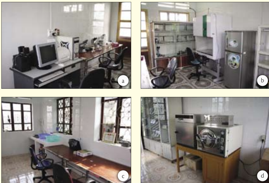
Figure 13.1 Typical arrangement of equipment in a diagnostic laboratory (laboratory in Nghe An PPSD): (a) and (b) two views of clean room, (c) and (d) two views of preparation room.
