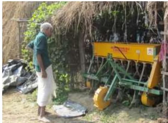
**Figure 6 Zero till machine provided by the project**
