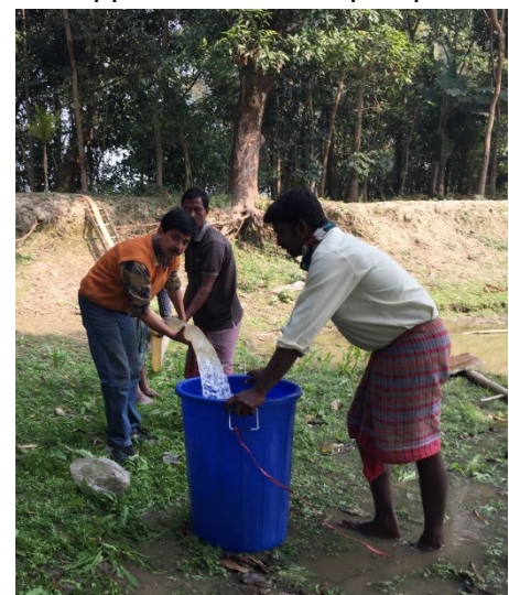
Figure 15 Bucket and Stopwatch method to collect pump discharge (flowrate) data
