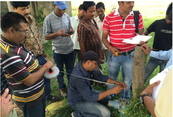
Figure 8 Using a low-cost method to measure depth to ground water table
