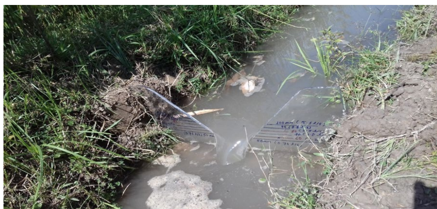
Figure 39 V-notch weir made from clear perspex installed in an earthen channel
