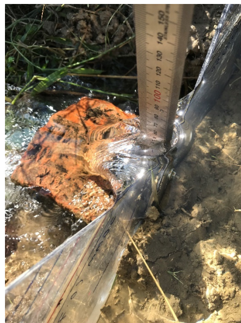
Figure 16 the depth of water flowing over a V-notch weir can be used to calculate the flow rate in a transfer channel
