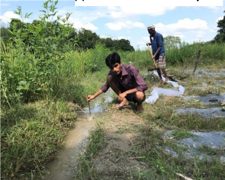
Figure 18 Measuring the discharge in a channel compared to the discharge from a polythene pipe
