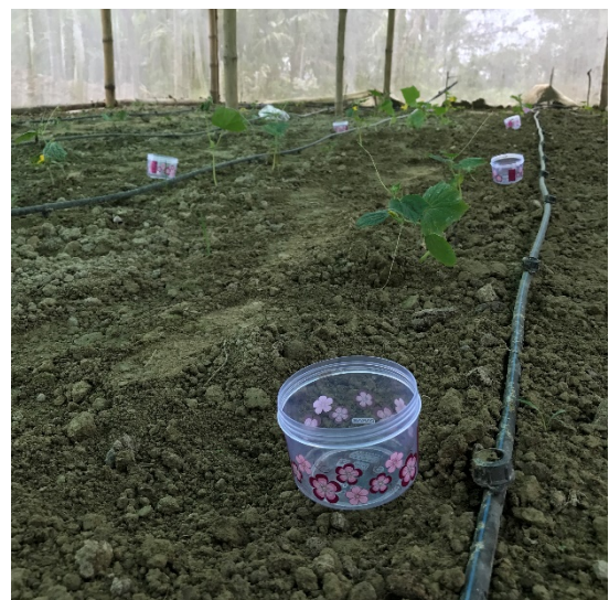
Figure 22 small plastic containers are used as catch cans to measure the uniformity of Drip irrigation
