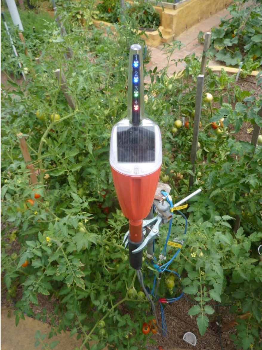
Fig 40. Current pre-commercial release of the Chameleon reader: this version is suited to continuous outdoor installation or for manually reading many installation sites.
